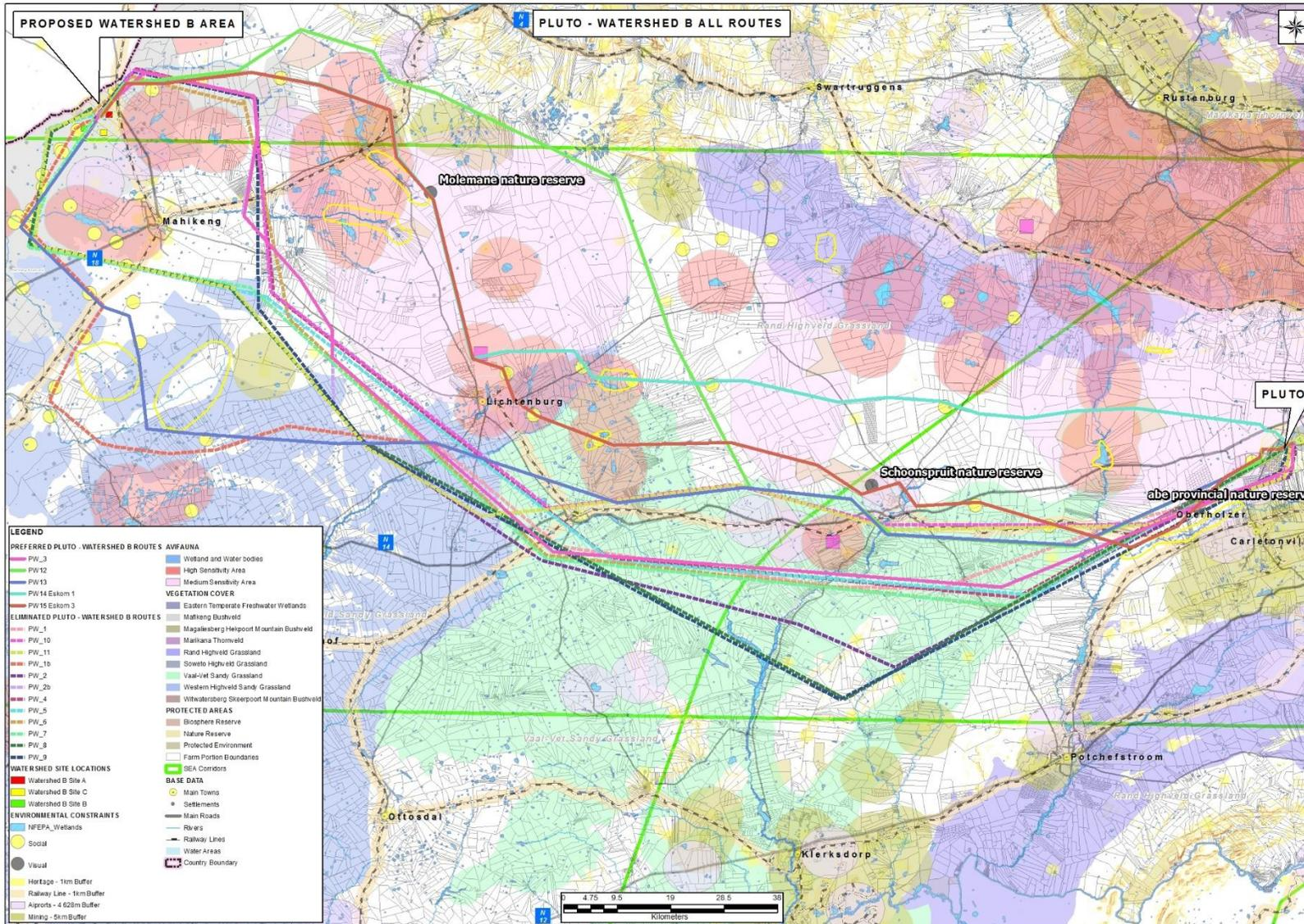
Figure 3. All route options between Pluto and Watershed B substation, based on the outcomes of the route screening process
